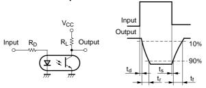
**Test Circuit for Frepuency Response**
