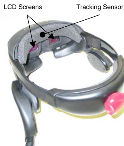
Figure 2: interior view of a HMD
