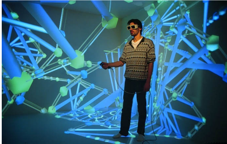
Figure 3: User in a CAVE wearing shutter glasses
