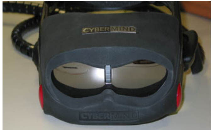
Figure 3: Frontside of HMD with adjustment wheel
