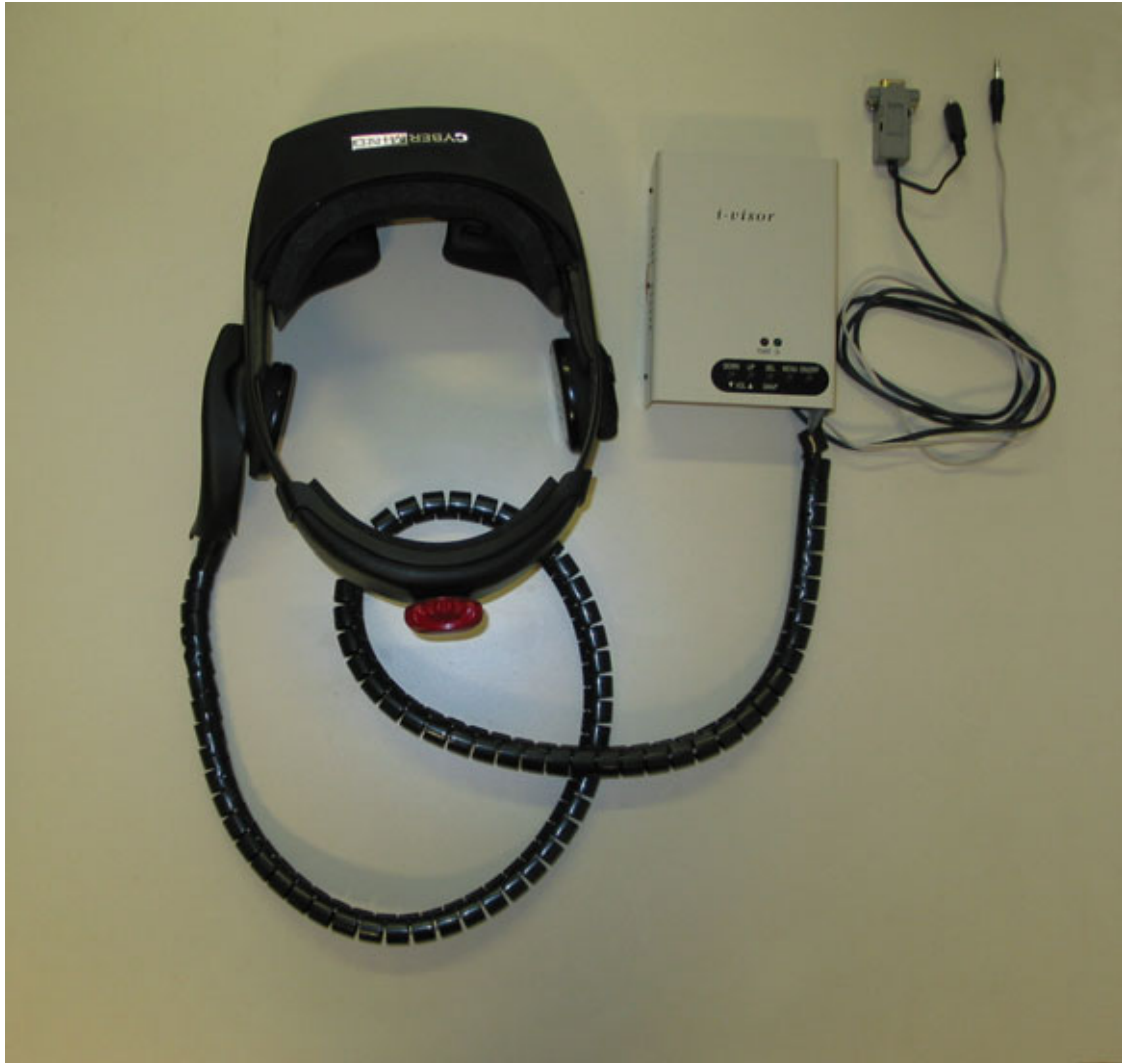
Figure 1: HMD, control unit, RS-232 connector and powercord for InterTrax 2 -tracker and audio input plug (from left to right)
