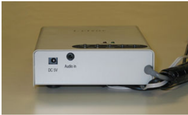
Figure 4: Frontside connections
