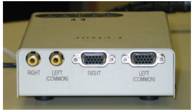
Figur 5: Rearside connections
