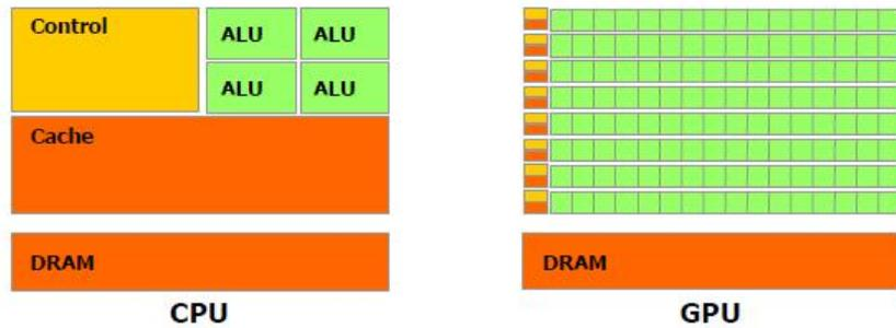
Figure 4.2. Layout of CPU and GPU architecture. Graph from [4].
