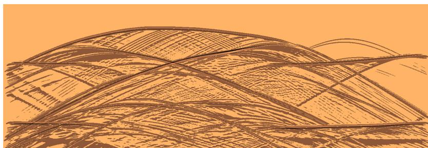
**Figure 2.8.** The seismic section after migration using a 1D velocity function.
