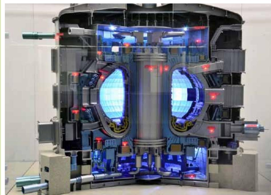
*This model of ITER, the world's largest tokamak, shows the doughnut-shaped vacuum vessel where the plasma is confined. The fuel — which is a mixture of deuterium and tritium, two isotopes of hydrogen — is heated to temperatures in excess of 150 million degrees Celsius, forming a hot plasma. Strong magnetic fields are used to keep the plasma away from the walls; these are produced by superconducting coils surrounding the vessel, and by an electrical current driven through the plasma.*
