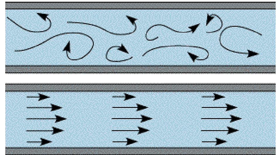
*The sketches show the difference between turbulent flow (top) and laminar flow (bottom) in a parallel channel. The arrows indicate the trajectory of particles in the fluid. As the particles in the turbulent case follow a more chaotic route, greater force is needed to keep the flow moving.*
