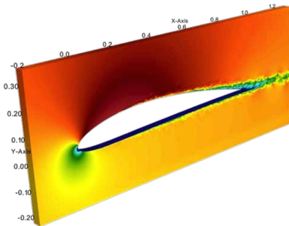
developing low-drag wing designs that reduce the area of turbulent air-flow and thus decrease the plane's fuel consumption and its impact on the environment.
