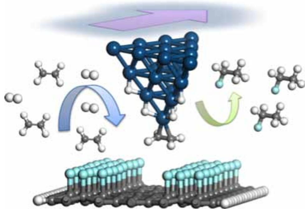
*Schematic diagram of the local reduction reaction of graphene fluoride via the cSPL technique with the assistance of a mixture of hydrogen and ethylene.*
