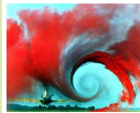
*The swirls above show a tip vortex formed behind the wing of a plane. The vortex has been made visible by having coloured smoke rising from the ground as the plane passes above it, so the smoke shows the air movement caused by the plane.*
