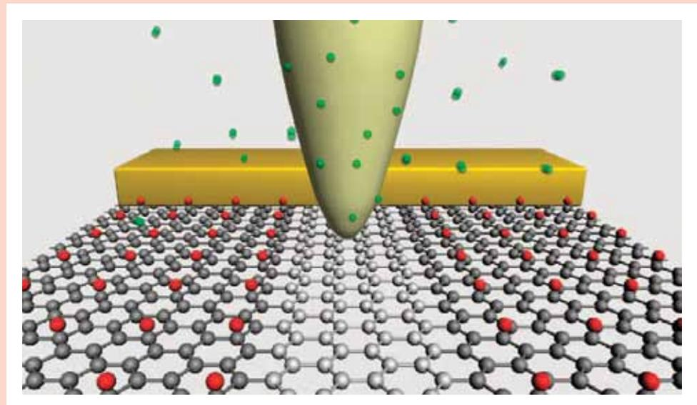
*Fluorographene is being turned into an electronic nanocircuit using the cSPL technique. A microscopic stylus with a chemical catalyst is moved across the surface of the fluorographene and reduces it chemically, so the fluorine is removed. This leaves a conducting graphene channel, which you can see in the centre. The channel connects to a metal electrode which is shown in yellow at the back.*
