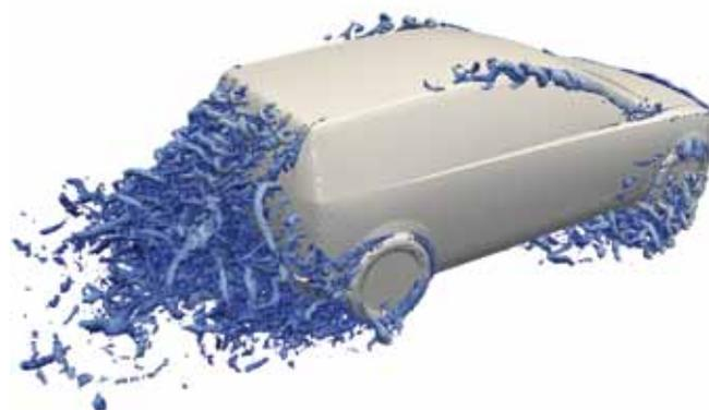
*Visualizations from a currently running simulation on Lindgren showing isosurfaces of Q-criterion for turbulent flow past a full car model, with geometry provided by Volvo. Simulation time is less than 48 hours using 1032 cores.*
