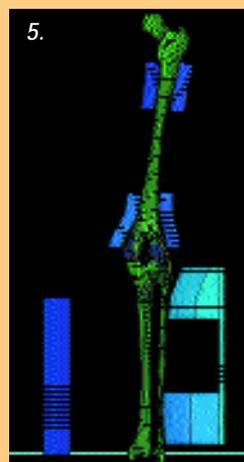
1. PAM-SAFE simulation of a pedestrian frontal knee impact, showing the knee joint.
