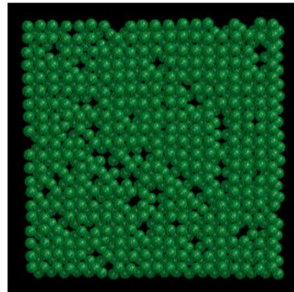
Distribution of voids in a structural layer of the bcc crystal.
