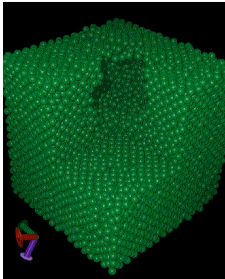
Fig. 1. A large-scale aggregation of vacancies in the fcc crystal.
