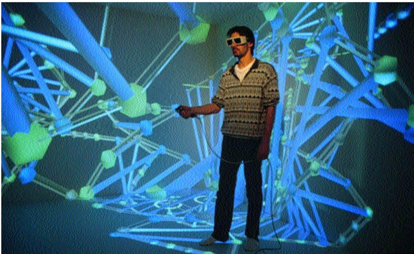
**Above:** Four of the Cube's six surfaces can be seen here, as well as the navigation wand and 3D shutter glasses.
