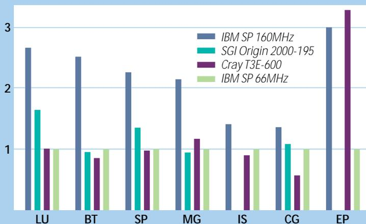
Fig. 2 Performance relative IBM SP 66MHz wide node for class C problems. Note: EP results are for 128 nodes.
