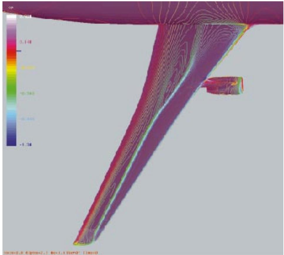
flow conditions are,  $Re/m = 11.16 \cdot 10^6$ ,  $\alpha = 2.2^\circ$  and  $M = 0.8$ .
