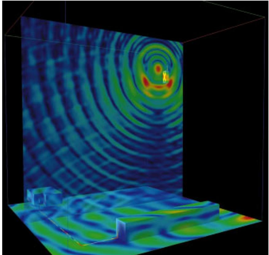
*A model setup for studying the induction of currents on a wire connecting two electronic devices in the presence of a transmitting cellular phone. The antenna on top of the telephone is driven by a current pulse and the picture shows a snapshot in time of the response. Execution time on the Fujitsu VX/2 at PDC was a few minutes and execution speed almost 900 MFlop/s.*
