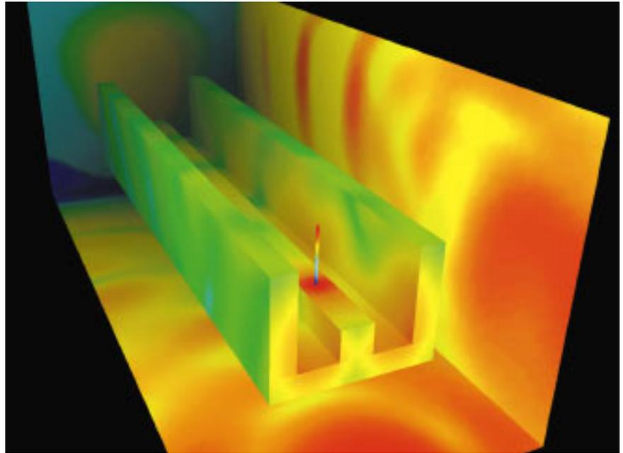
*This figure shows, for a distinct time, the solution of an open waveguide problem. An antenna is attached to an E-shaped waveguide and a current pulse is injected into the antenna.*
